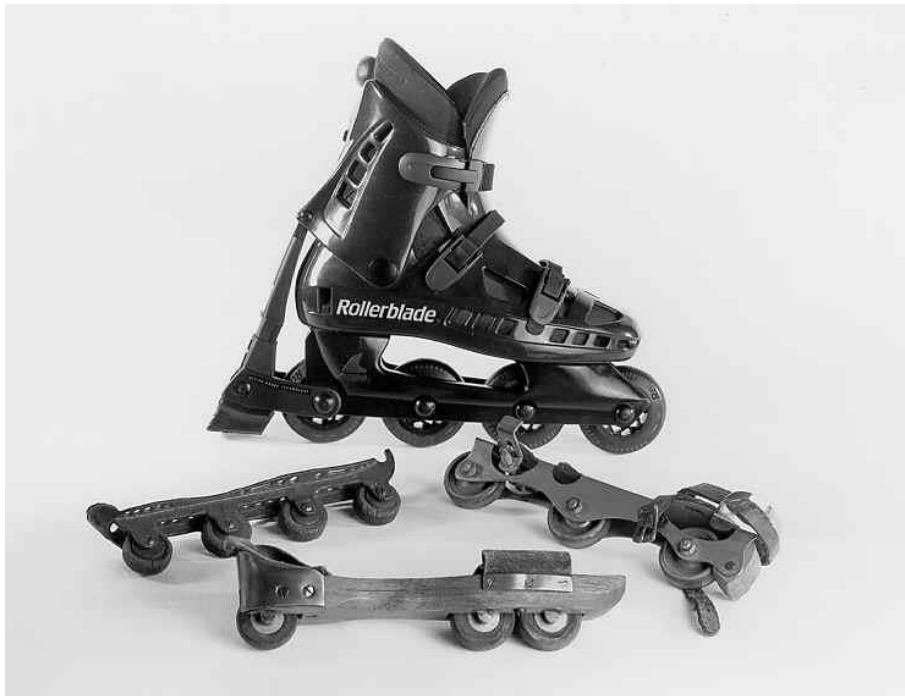
Figure 2 – A selection of in-line roller skates through the ages (www.rollerskatingmuseum.com, 2001). Clockwise from top: A 1994 Rollerblade Inc. skate, 1930’s Best-Ever-Built Skate Company clamp on skate, an 1819 Petittbled skate, a skate of unknown origin circa 1860.
